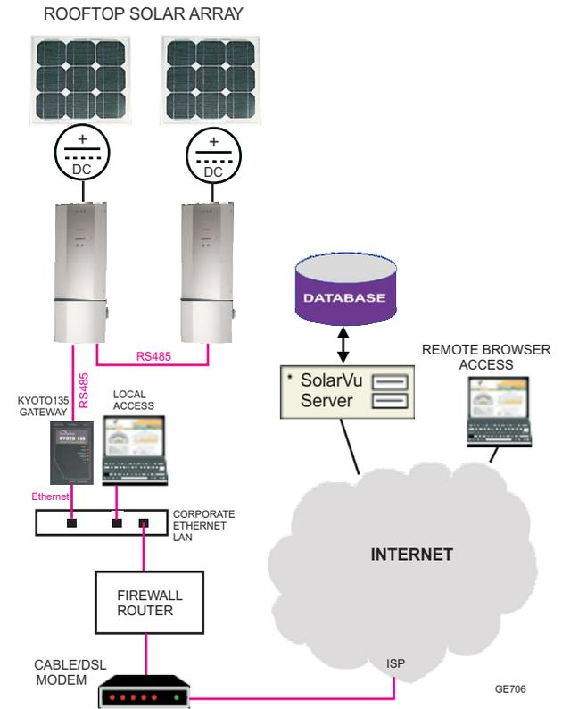
Fig 2 K135-KACO XP10U RS485 connections
