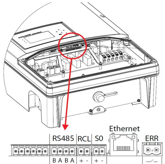
\* Program unique slave address using Menu Level 1 - Interface Set Bus Termination = ON for last inverter in string only
