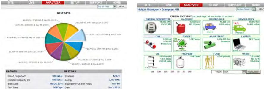
Fig 11 View power and energy now or output for any time period on the LIVE screen.
